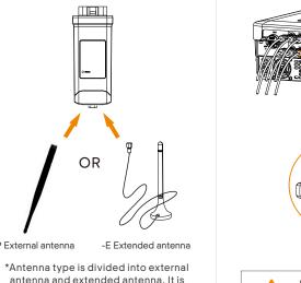
> Plug the Pocket WiFi into the correct port of inverter.
